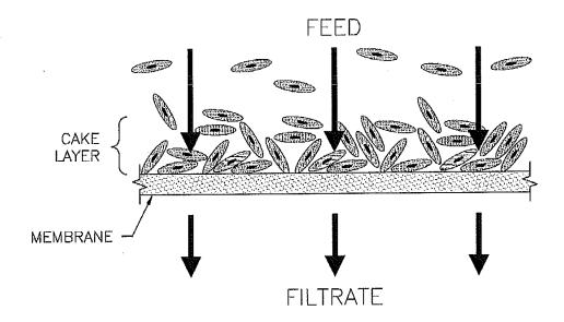
Most hollow-fiber MF and UF systems operate in deposition mode. Typically, accumulated solids are removed from MF/UF systems by backwashing. However, some systems operate until accumulated solids reduce the flow and/or TMP to an unacceptable level, at which point the membrane cartridge is replaced.
